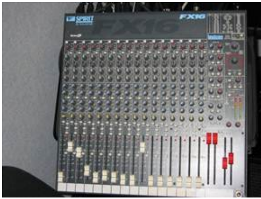
Figure 9. Soundcraft FX 16 sound mixer
