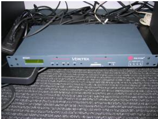
Figure 10. Polycom Vortex 2241 echo-canceling unit
