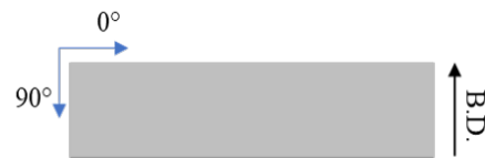
Figure 3. Residual stress measurement directions. The building direction is indicated by a black arrow.
