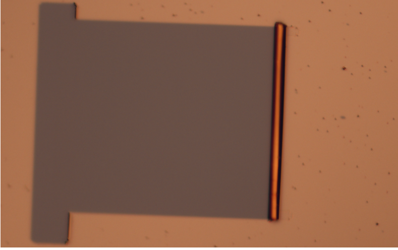
Figure 3.5 Optical microscope image of SiO 2 /Au based RUTs fabricated using Ge as a sacrificial layer.
