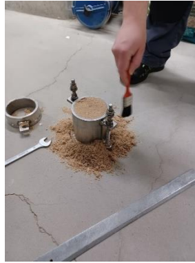
Figure 49. Result after compaction and flattening
