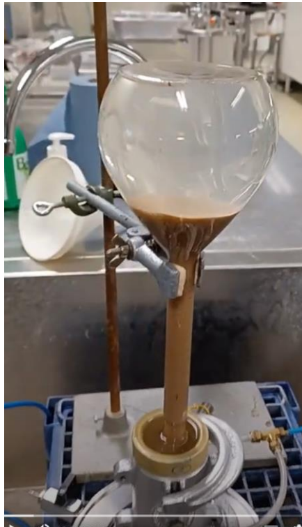
Figure 52. Wet pluviation set-up with flask
