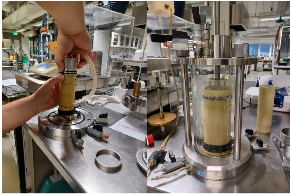
(a) (b) Figure 51. Preparing the sample and triaxial cell
