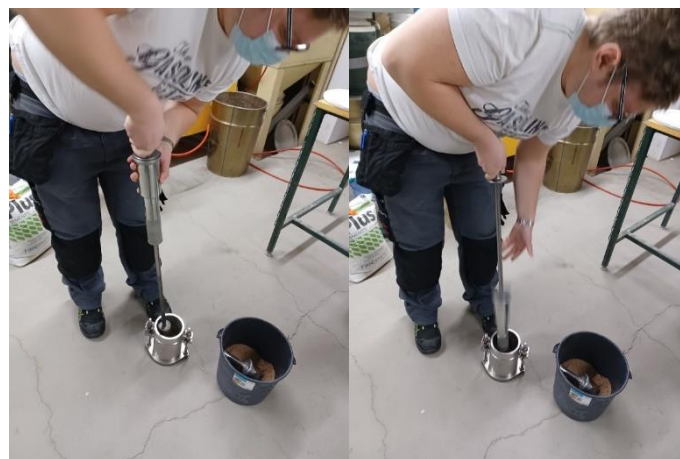
Figure 48. Compacting the sample
