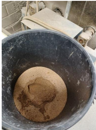
Figure 47. Moistening of the sample
