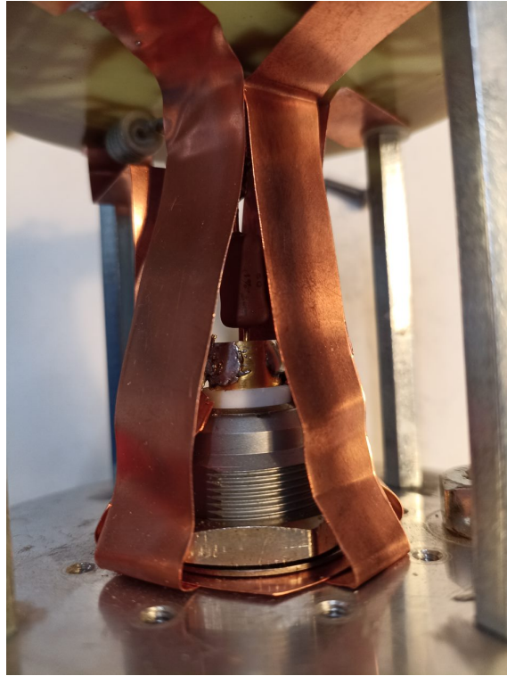
Figure 4.2. New LVA with loop size minimized.
