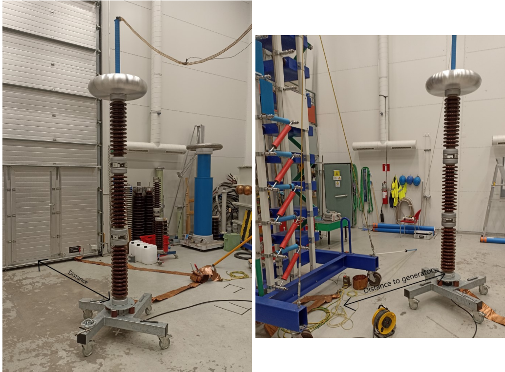
Figure 5.3. Test setup for measuring the proximity effect.
