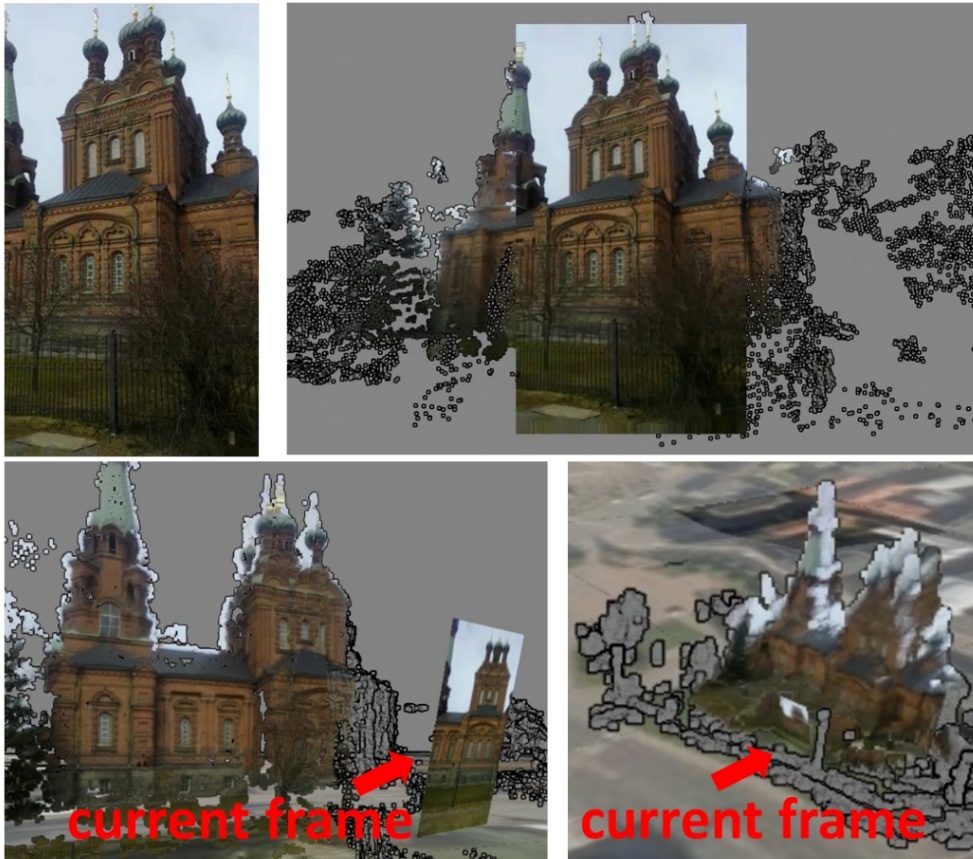
Figure 5.3 A few different video playback options are illustrated. Ordinary video playback mode (upper left): video is played back as same as the captured video; Expanded view mode (upper right): user can expand their field of view to surrounding environments that are not visible in the original video frame by the augmented 3D model; Motion trajectory (bottom left): with the scene fixed and see camera's trajectory along the scene. Bird-view (bottom right): users can arbitrarily change their viewing angles, and see the scene in an aligned and augmented map.
