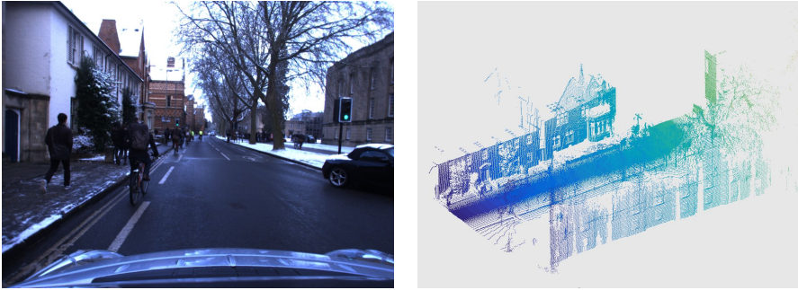
Figure 2.7 A street-view snapshot (left) and a LIDAR point cloud (right) from the Oxford RoboCar Dataset [82].
