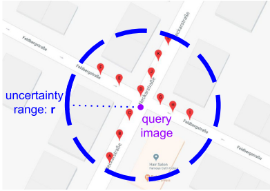
Fig. 5. Single-reference pose estimation. The actual location of the query image is marked with a purple dot, and a circle around the purple dot represents the initial uncertainty on the location of the query image. Within the uncertainty circle, one reference image is randomly selected among all possible candidates that are indicated with red markers from A to L. (For interpretation of the references to color in this figure legend, the reader is referred to the web version of this article.)
