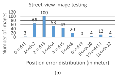
Fig. 5. Histogram of orientation errors and the position errors for 305 street-view images.
