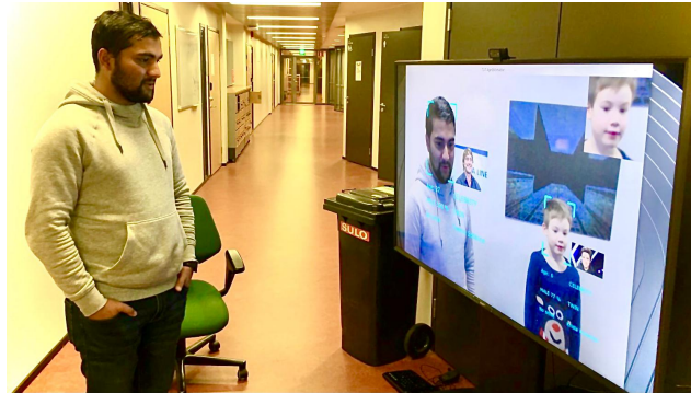
Fig. 1. Our real-time facial recognition system in action. It detects human faces on a frame captured by a webcam, recognizes age, gender, and emotion in real-time. Additionally, it shows the most similar appearing face obtained from the similarity search network.
