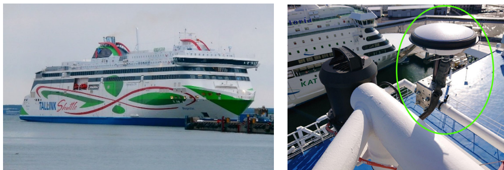
Figure 2. MS Megastar [23] cruise ship (left), GNSS antenna installed on the top mast of the vessel marked within green ellipsoid (right).
