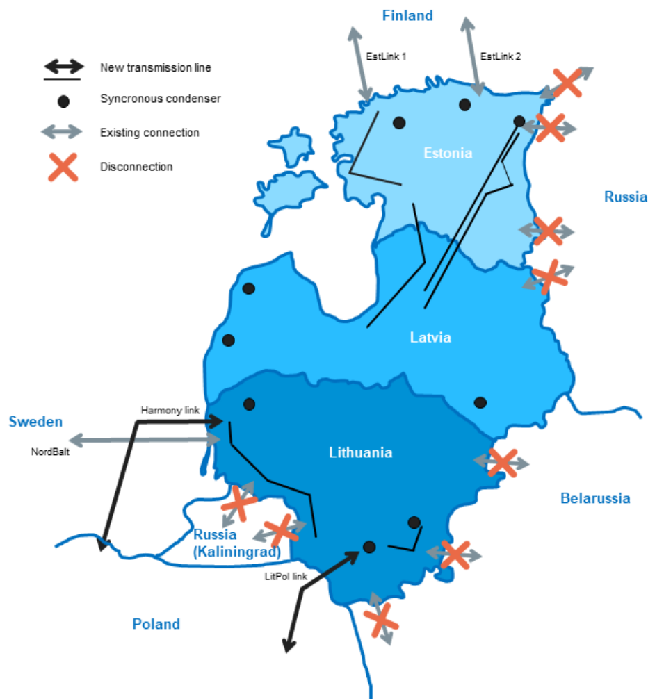
Figure 12. Baltic synchronization plans with the Continental European grid in 2025 with planned decommissioning, new interconnectors and planned and implemented grid reinforcements [49].
