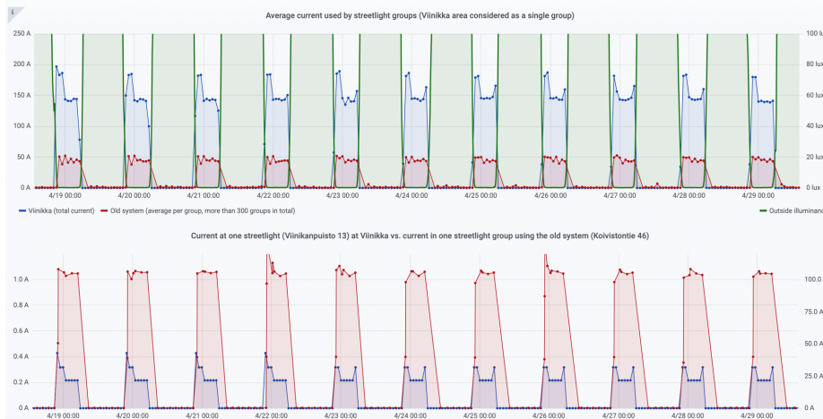
Figure 6: Visualization of average electric current in streetlights using Grafana.
