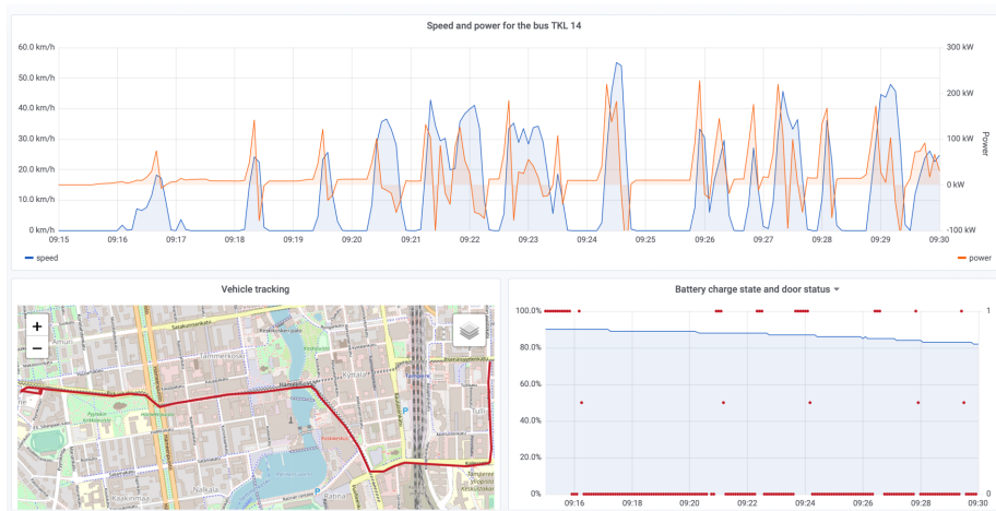
Figure 8: Visualization of speed and power, location, battery charge, and door status for a Tampere City electric bus using Grafana.
