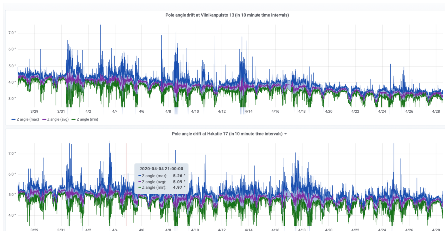
Figure 7: Visualization of pole angle drift of two streetlights using Grafana.
