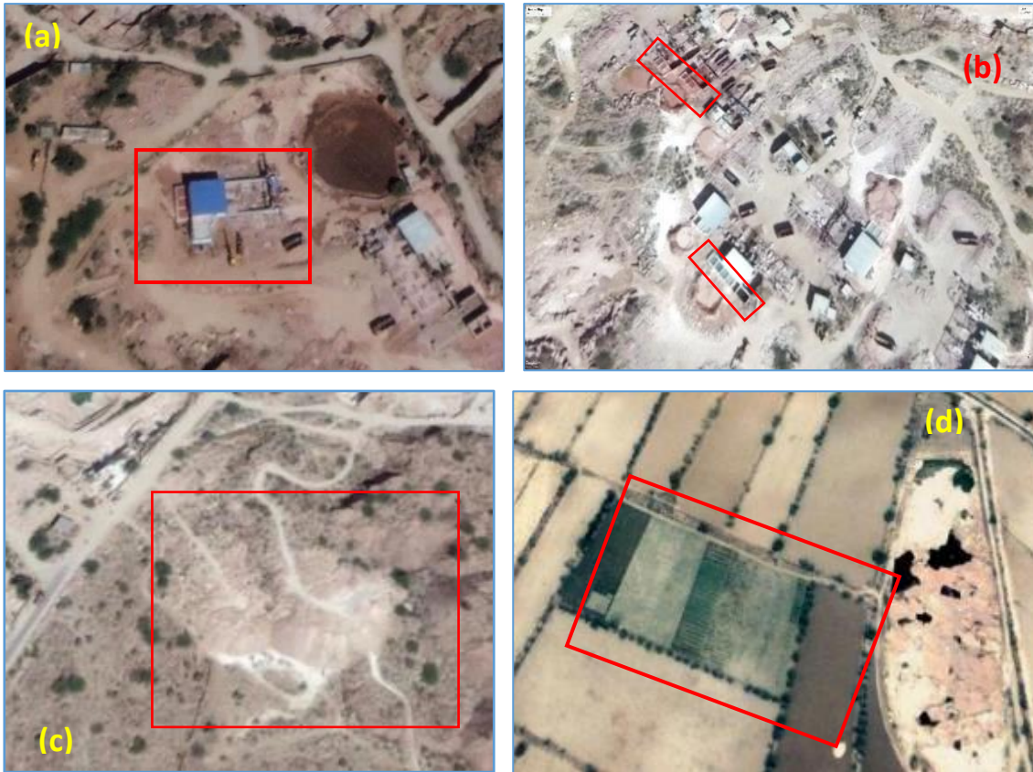
Fig 3. (a) Satellite image of a cutting unit; (b) satellite image of water recovery ponds for slurry from cutting units; (c) satellite image of dumps used for disposing slurry and (d) satellite image of agricultural land with crops near the quarrying area.
