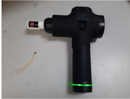
Fig. 4 Energy harvester connected to muscle maintenance hammer
