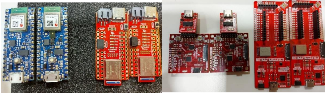
Fig. 13 Boards from left to right: Arduino Nano 33 BLE and Arduino Nano 33 BLE Sense, two Artemis Nano, two Edge and two Artemis DK boards.
