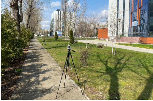
Fig. 2. Location at which the range of the devices was measured. The devices were placed at distances between 5–220 m along the pathwalk.
