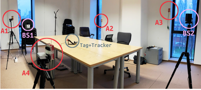
Fig. 8. Localization setup: the four anchors (A1 to A4) encompass an area of approximately 4.5 \times 3.6 m and the tracking area is on the table. The ground truth was acquired using two HTC Vive base stations (BS1 and BS2) and a tracker that was collocated with the UWB tag, shown on the table.
