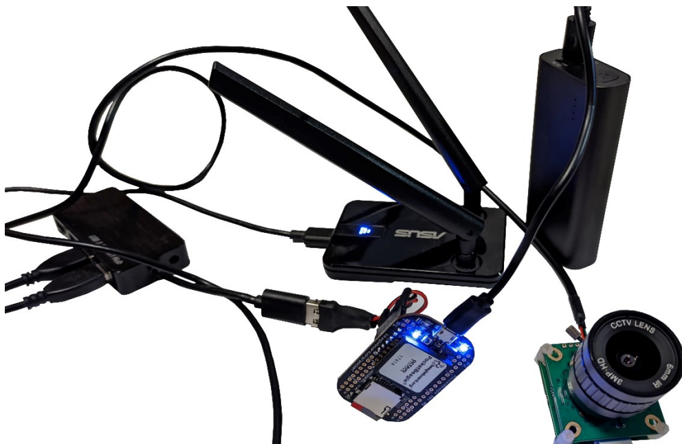
Figure 2 –The embedded platform with a USB hub, the camera, a WiFi module, and a battery pack connected.
