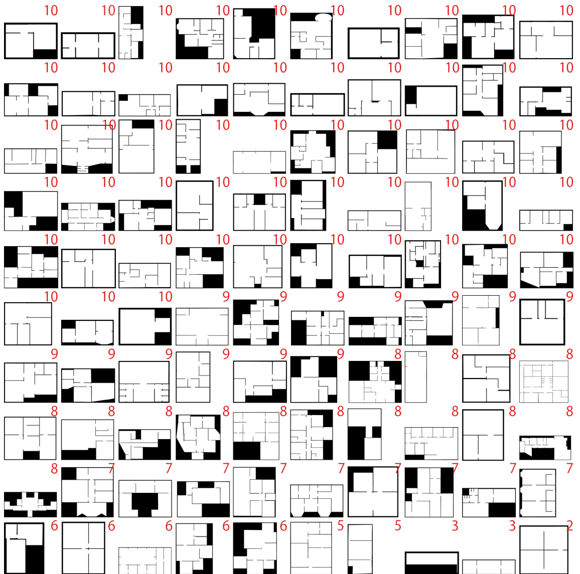
Figure 4.1. All of the tested maps with the number of test runs where the robot was localized successfully for each map.
