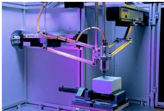
Figure 8: The Orthoglide (© CNRS Photothèque / CARLSON Leif)
