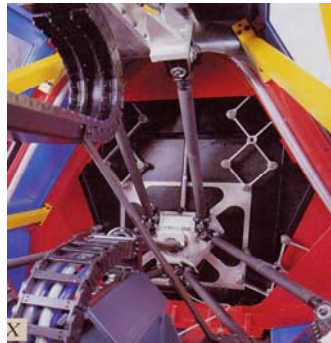
Figure 14. Urane SX tool is isolated from the mechanism that generates the motion (from "Renault Automation Magazine", n° 21, may 1999)
