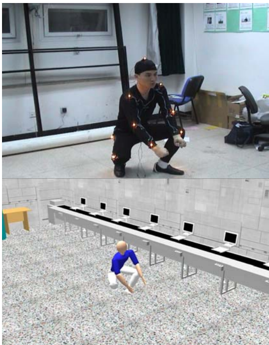
Fig. 4 Tracking result in the simulation software. The upper one shows the action of worker and the same action of the virtual human in the simulation software in the lower one.
