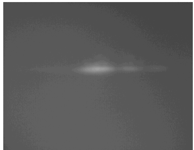
Fig. (14). Near-field photo of intensity in P3OT buried waveguide at 1550 nm.
