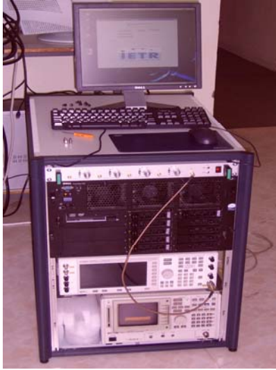
Fig. 3 Receiving and acquisition system
