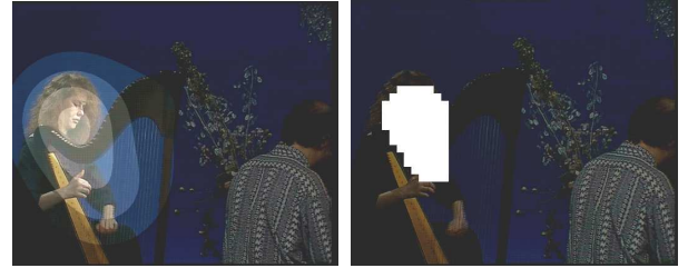
Fig. 3. Saliency map (left) and the resulting macroblock-based RoI (right) of Harp sequence.
