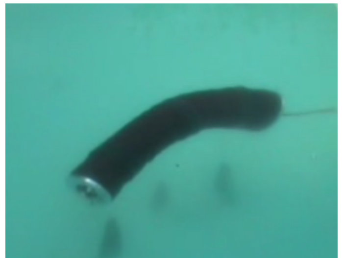
Figure 17. PICTURE OF A 6 VERTEBRAE IN A SWIMMING POOL TO TEST THE WATERTIGHTNESS AND BUOYANCY
