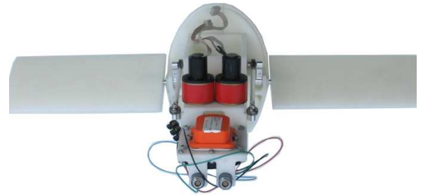
Figure 13. PROTOTYPE OF THE HEAD MADE IN RAPID PROTOTYPING WITH TWO CLOSED-LOOP CHAINS TO CONTROL THE FINS
