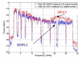
The input impedance has not been yet modified and the transmitted OFDM waveform is not EMC compliant. We can observe that HD-PLC presents deeper notches than HPAV with a less emission power. We can notice that it is not possible to use the two protocols at the same time as they have non-interoperable PHY layers.
