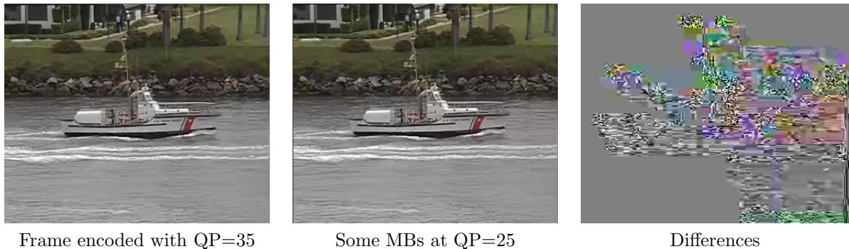
Figure 5. Differences between a frame encoded with QP=35 and the same in which some MBs are encoded at QP=25.
