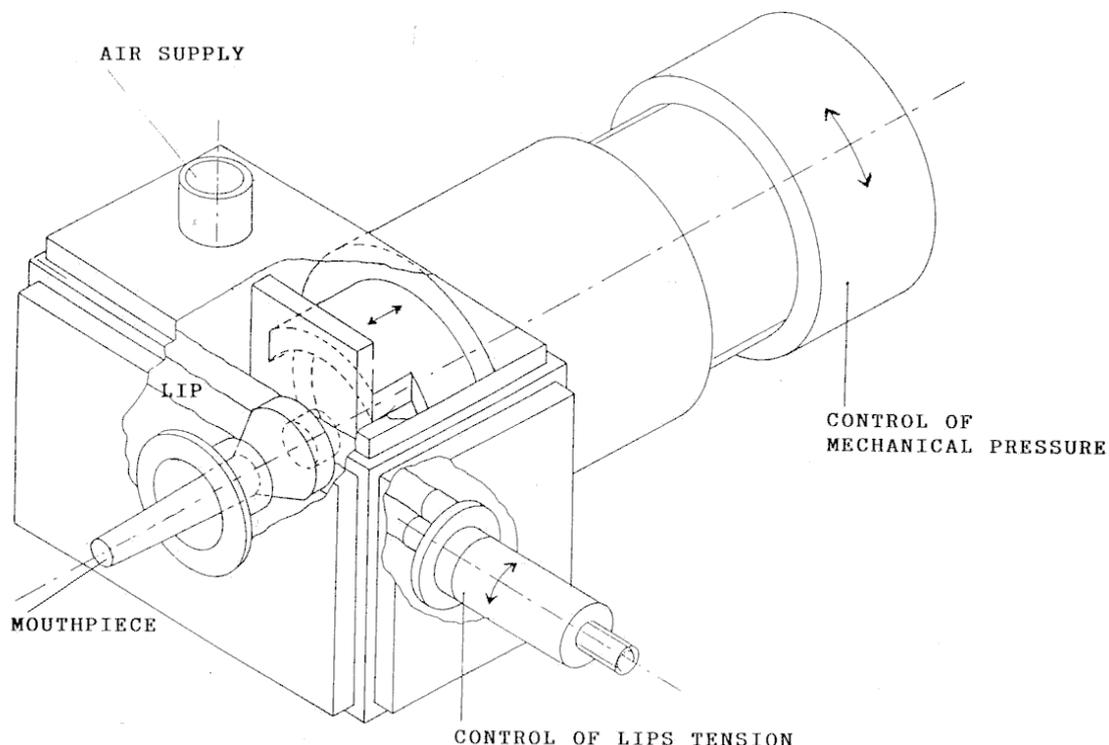
**Figure 1.** *Artificial mouth for brass instruments (version #2).*
