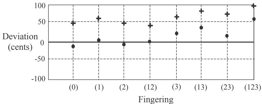
**Figure 4:** Compared intonation accuracy of the 3rd resonance frequencies of a trumpet (o) and the 3rd regimes played by a trumpet player (+) corresponding to the 8 fingerings. The intonation accuracy is defined as the deviation in cents of the analysed frequency (resonance frequency or playing frequency) relatively to an ideal location (based on the equally tempered scale with  $A_4=440\text{Hz}$ ).
