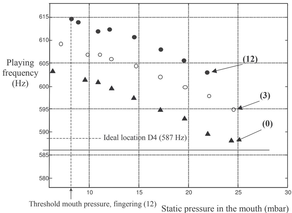
**Figure 7.** Variation of the playing frequency for three fingerings of the trumpet Y for the D4 played using the artificial mouth, with increasing mouth overpressure. The three different fingerings are:
