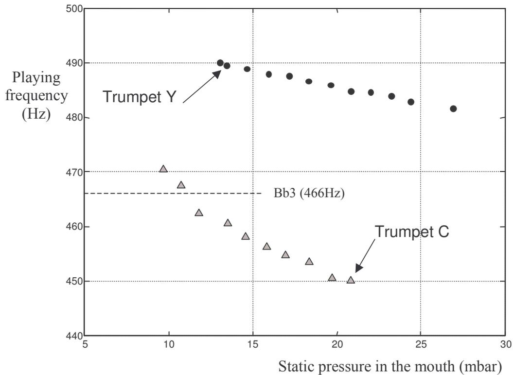
**Figure 5.** Evolution of the playing frequency for the same fingering, for two trumpets C and Y. Bflat3 is played with the artificial mouth with the same embouchure. The playing frequency (in Hz) is represented according to the mouth overpressure (in mbar).
