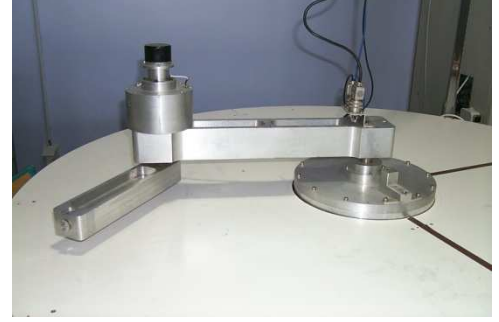
Fig. 5: The scara robot prototype.
