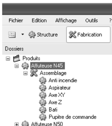
Figure 11: Manufacturing decomposition of a grinding machine
