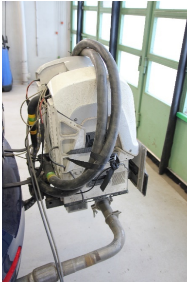
175 Figure 1: Portable emission measurement (PEMS) device installed on a test car.
