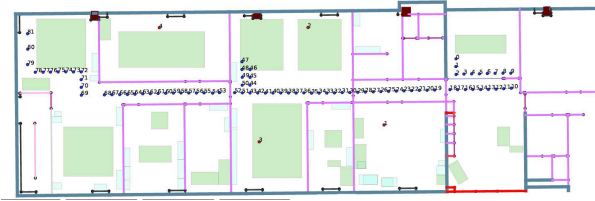
Fig. 9. Measured CIR along indoor selected trajectory, (red points) 4 Tx (1 is bottom right), (blue points) 81 Rx (0 right - 81 right)
