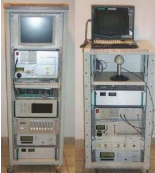
Figure 1. MIMO channel sounder: receiver (left) and transmitter (right)
