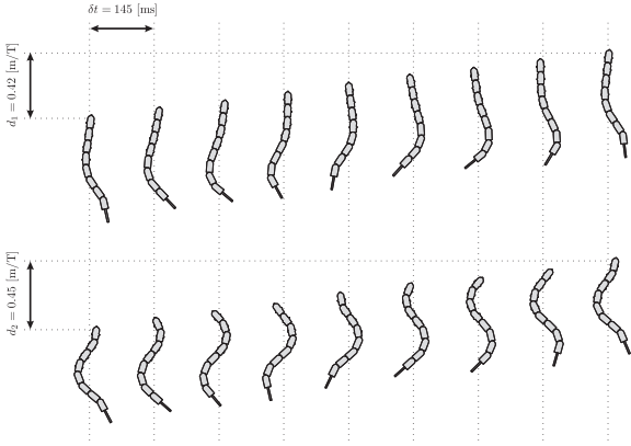
Fig. 2. Representation of AmphiBot’s configuration for two swimming gaits, with: linear ramp of joint amplitudes from \alpha_1 = 0\text{deg} to \alpha_7 = 35\text{deg} , (top); uniform joint amplitudes \alpha_i = 35\text{deg} , i = 1, \dots, 7 , (bottom); with parameters \eta = 1 , \nu = 0.85\text{Hz} .
