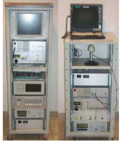
Figure 1. MIMO channel sounder: receiver and transmitter..
