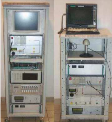
Fig. 1. MIMO channel sounder: receiver and transmitter.
