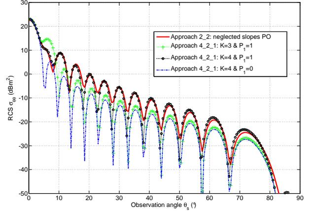
Fig. 4. Bistatic RCS at 5 GHz of the selected surface made of 1 cosine calculated with the “numerical neglected slopes PO” approach and analytical cosine approach 4\_2\_1 for different summation indexes values.
