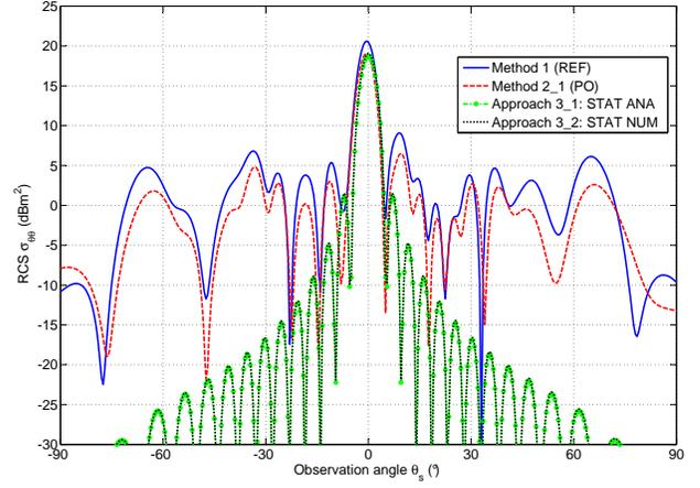
Fig. 2. Bistatic RCS of Sample 2 at 5 GHz, at normal incidence and in  $\theta\theta$  (or VV vertical-vertical) polarization, computed from: Method 1 (FEKO MLFMM used as reference), Method 2\_1 (numerical PO), Approach 3\_1 (analytical statistical) and Approach 3\_2 (numerical statistical).
