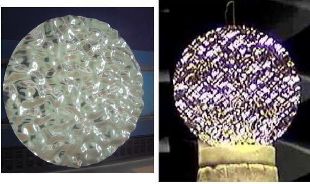
Fig. 7. Built surface samples, on the left: sample 3 (Gaussian autocorrelation function,  $L_c = 3$  cm), on the right sample 2 (exponential autocorrelation function,  $L_c = 5$  cm) mounted on the Styrofoam mast in the measurement chamber.
