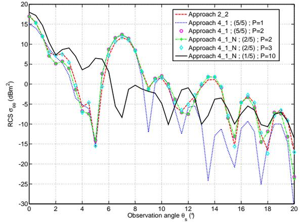
Fig. 6. Monostatic RCS at 5 GHz of the selected surface made of 5 cosine components calculated with the “numerical neglected slopes PO” approach and Approach 4\_1 for different summation indexes  $P$  and different numbers of constitutive cosine components accounted for in the calculation.
