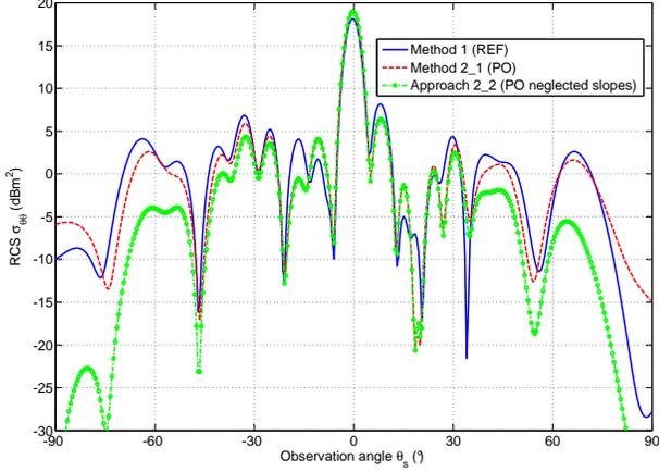
Fig. 3. Monostatic RCS of Sample 3 at 5 GHz and in  $\theta\theta$  polarization calculated by: Method 1 (FEKO MLFMM used as reference), Method 2\_1 (numerical PO) and Approach 2\_2 (“numerical neglected slopes PO”).
