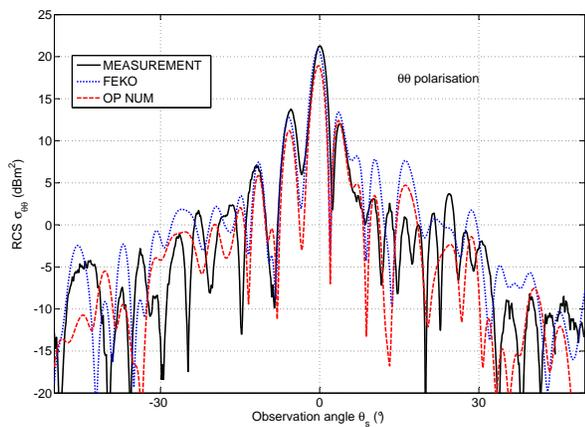
Fig. 12. Rough surface sample 2 RCS in  $\theta\theta$  polarization, and at 5 GHz.
