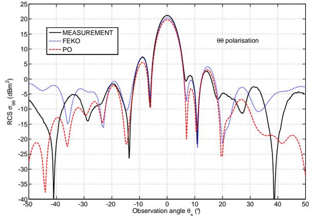
Fig. 10. Rough surface sample 3 RCS in  $\theta\theta$  polarization, and at 2 GHz.
