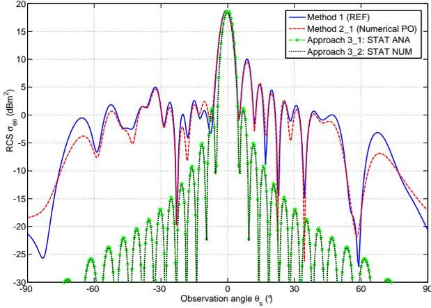
Fig. 1. Bistatic RCS of Sample 1 at 5 GHz, at normal incidence and in  $\theta\theta$  (or VV vertical-vertical) polarization, computed from: Method 1 (FEKO MLFMM used as reference), Method 2\_1 (numerical PO), Approach 3\_1 (analytical statistical) and Approach 3\_2 (numerical statistical).
