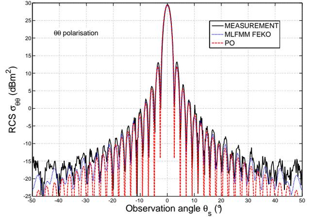
Fig. 9. Smooth plate RCS and phase in  $\theta\theta$  polarization at 5 GHz.
