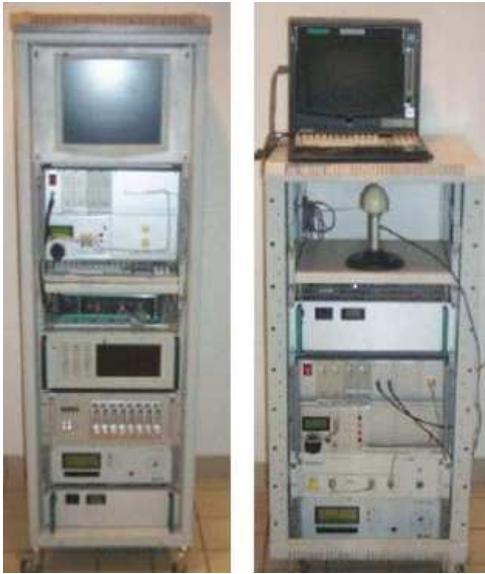
Fig. 2 MIMO channel sounder: receiver (left) and transmitter (right).
