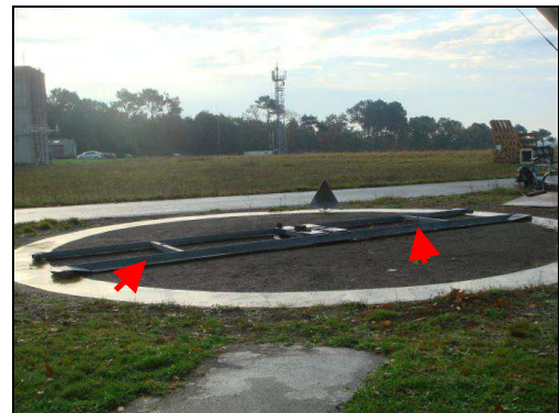
Figure 1 - The rotating steel platform used in the RCS measurement in the outdoor conditions
