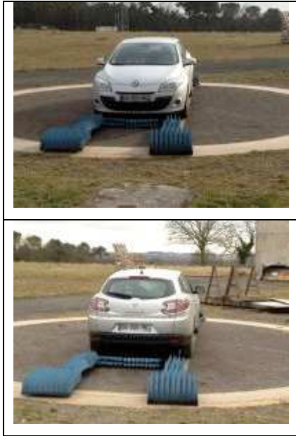
Figure 2 - The rotating steel platform is protected by microwave absorbers in the front and the rear of VUT
