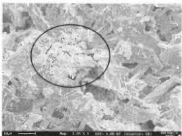
Fig. 5. Modification of the plaster phases versus temperature at 20, 100 and 300°C (DRX – SEM), G: gypsum, H: hemihydrate, A: anhydrite
