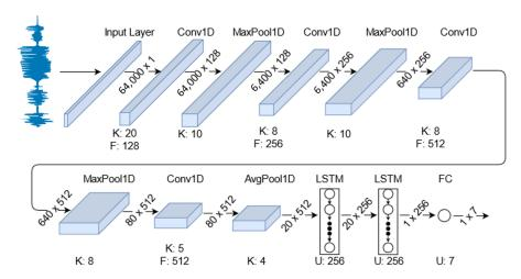
Figure 2. The architecture of the proposed 1D CNN + LSTM-based deep neural network.
