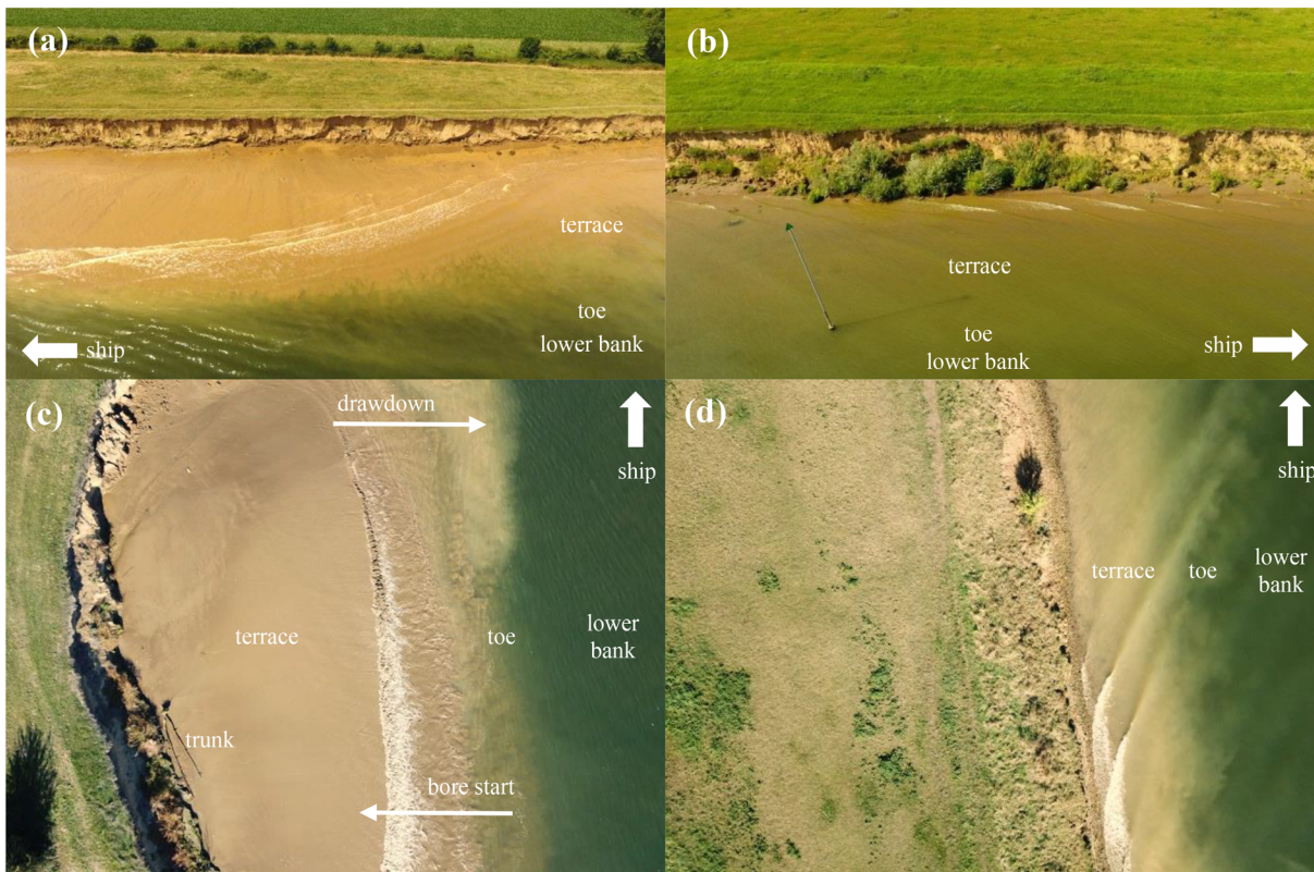
Figure 4. (a) Primary wave propagating over terrace as secondary waves break over it, km 153.9 on 21 June 2017. (b) Secondary waves breaking near the upper-bank toe, km 153.5 on 23 August 2017. (c) Primary wave ejecting sediments from terrace, km 153.6 on 10 October 2018. (d) Secondary waves breaking at upper-bank toe over gravel layer, km 154.3 on 10 October 2018.
