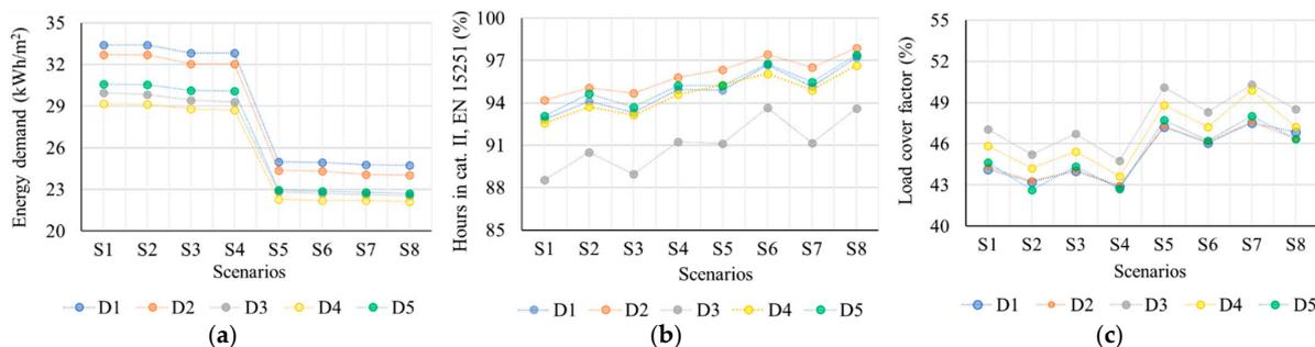
**Figure 4.** Results of the three performance indicators for the five analysed designs across the eight scenarios: (a) Energy demand results (including only heating, cooling, and lighting). (b) Thermal comfort results (average % of hours in cat. II of EN 15251 in five main rooms). (c) Load cover factor results.
