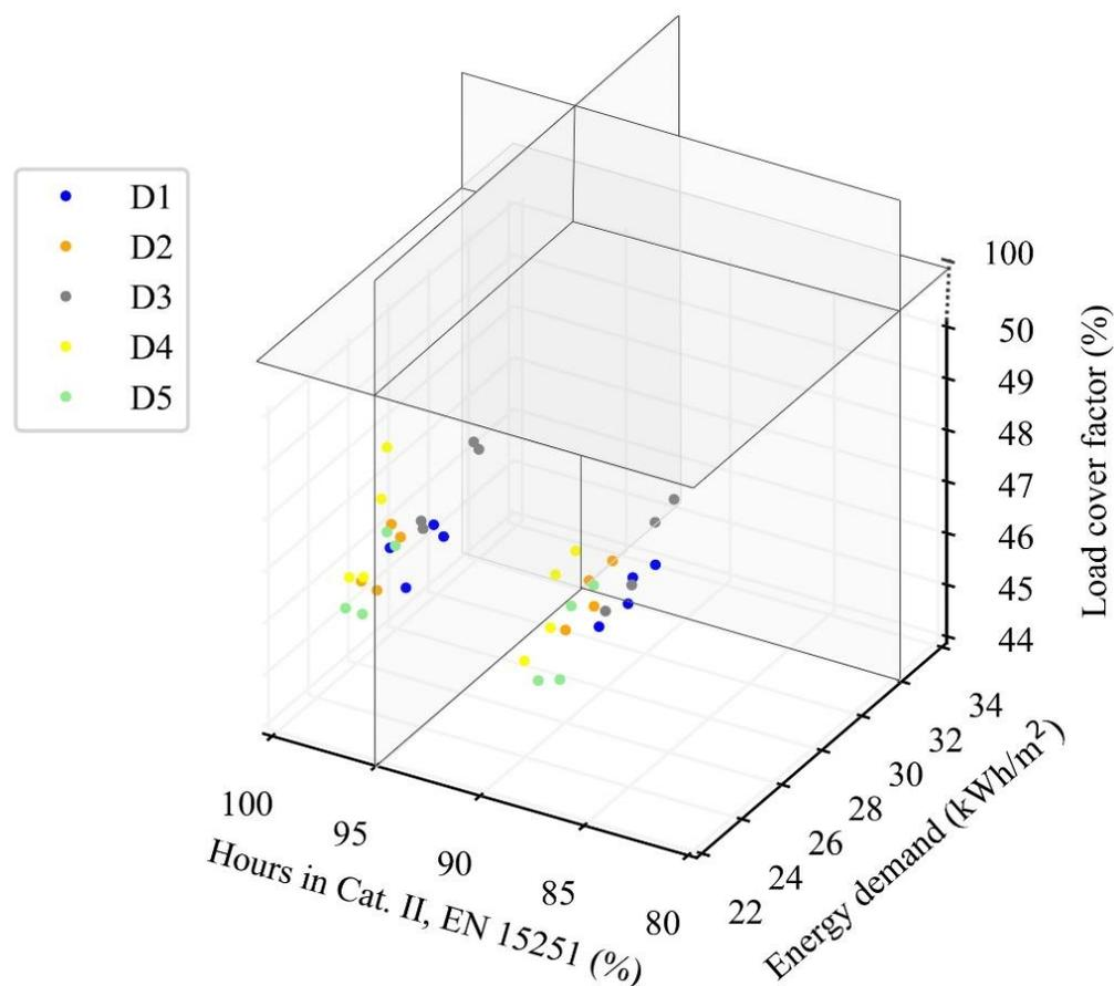
**Figure 6.** Energy demand vs. percentage of hours in Category II of EN 15251 vs. load cover factor, for the five designs across the eight scenarios. The three highlighted planes show the robustness margins for each indicator.
