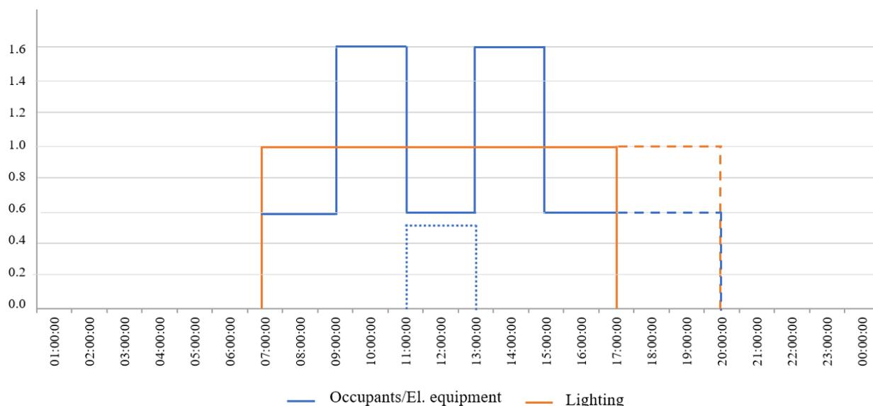
**Figure A1.** Profile schedules used for occupancy, electric equipment, and lighting in the analysed scenarios. \* The dashed blue and orange lines denote scenarios 2, 3, 7, and 8, which imply a longer stay of occupants in specific rooms. \*\* The dotted blue line denotes the occupation profile for the canteen, which is the only zone whose occupation differs from the rest of the modelled zones.
