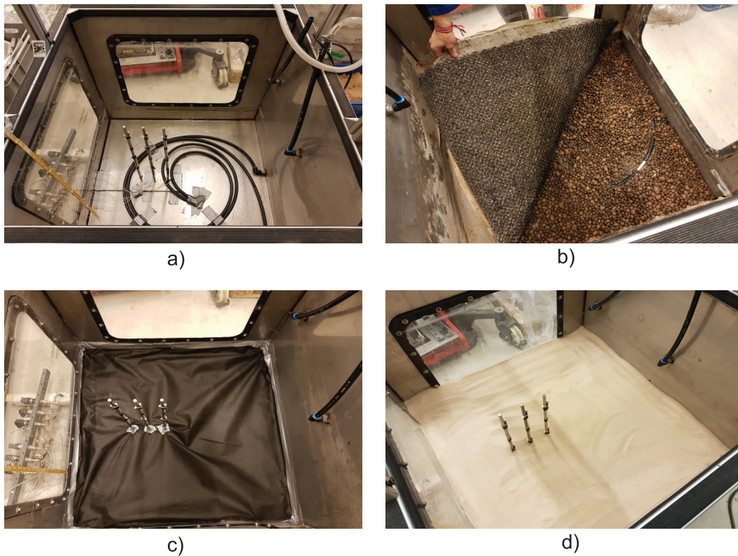
Fig. 4. Stages in initial soil model preparation: (a) support for pore pressure standpipes and perforated tubes for saturation and drainage of soil model; (b) filter layer (LECA and geotextile); (c) geotextile as separation layer; (d) filling of dry sand. [Colour online.]
