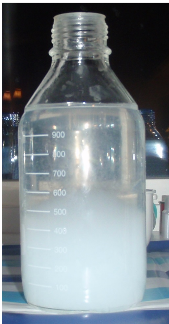
Figure 2-10. A container with 1000 mL seawater that was mixed with 10 mL 50% NaOH solution. The white solids are precipitation of magnesium and calcium. This home experiment was executed by Ivar Ervik.
