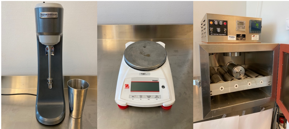
Figure 2-1: Hamilton Beach Mixer to the left, Ohaus Pioneer Precision PX3202 in the middle, Ofite roller-oven #172-00-1-C to the right.
