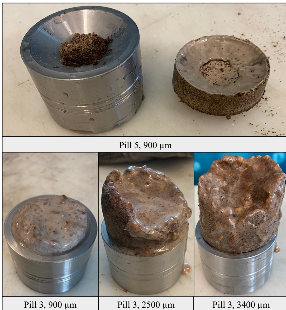
Figure C-2: Tapered discs after pressure tests for pills with no \text{CaCO}_3
