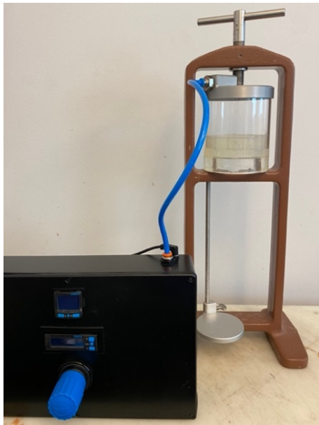
Figure 2-8: Festo Pressure regulator LRP-1/4-2.5 and LRP-1/4-0.25, Festo Pressure Sensor SPAN-PO25R and SPAN-P10R, Festo Flowmeter SFAH-10U, cell for disc insert.
