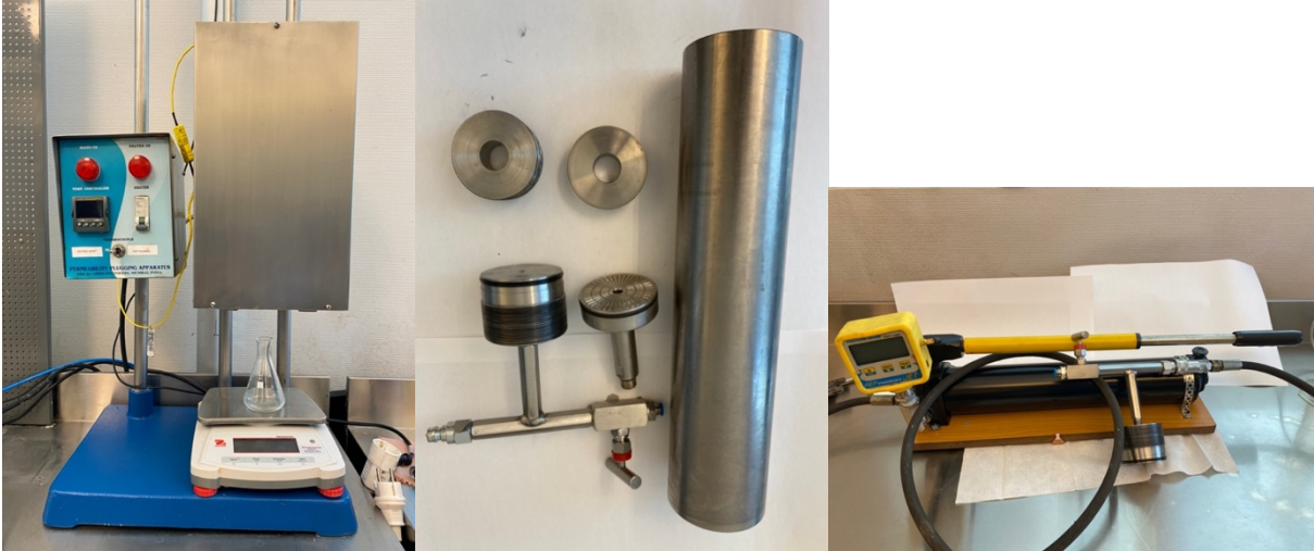
Figure 2-10: Permeability Plugging Apparatus to the left, main parts of the insert in the middle, pressure and logging device to the right.
