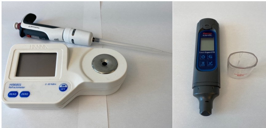
Figure 2-9: Hanna Instruments Sucrose Refractometer HI 96801 to the left, Eutech Expert CTS to the right.
