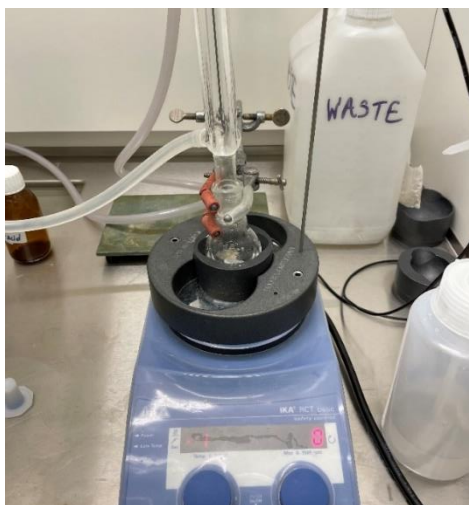
Figure 4.1. Synthesis setup for MIP-202, using a round bottom flask with a stir bar and a reflux condenser on a hot plate.
