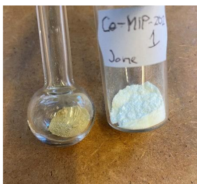
Figure 5.9. Ce-MIP-202-04 sample in an analysis cell before (right) and after (left) degassing at 120°C.
