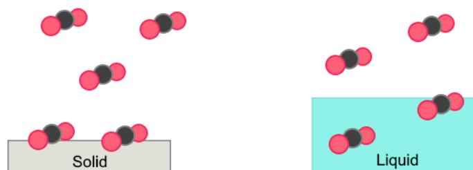
Figure 2.1. Comparison of the mechanics CO 2 adsorption has onto a solid surface (Left) and the absorption of CO 2 molecules into a bulk liquid (Right)
