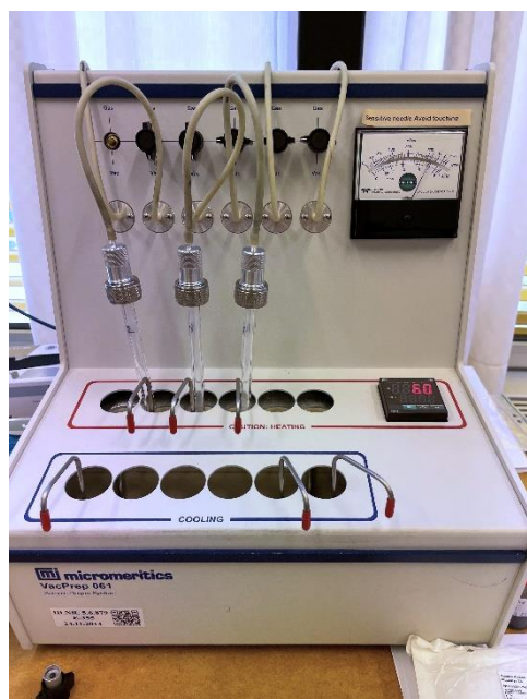
Figure 4.2. Micromeritics VacPrep 061 Vacuum Degas System with three sample cells under degassing at 60°C.
