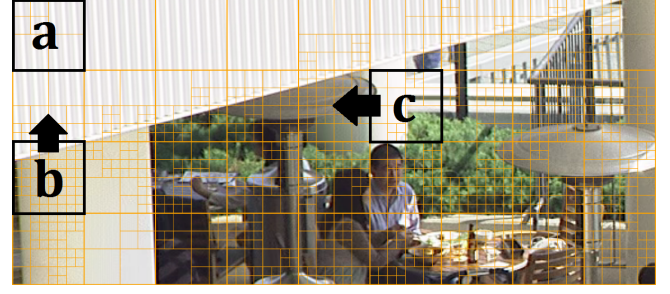
Fig. 3: Different possible prediction configurations, a \Rightarrow predictor, b \Rightarrow above CTU, c \Rightarrow left CTU.
