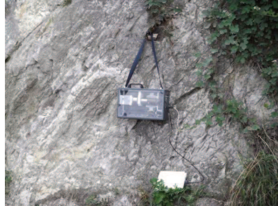
Figure 4.2: Field measurement using the CavaRad detector.
