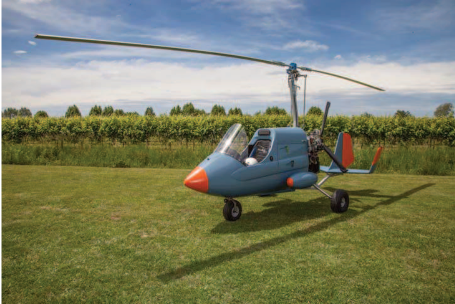
Figure 5.1: Picture of the Radgyro, the autogyro dedicated to multi-spectral airborne acquisitions, used for the AGRS surveys over the sea.
