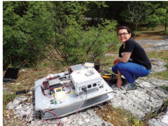
(b) Acquisition of a ground calibration measurement with the AGRS_16L detector.
