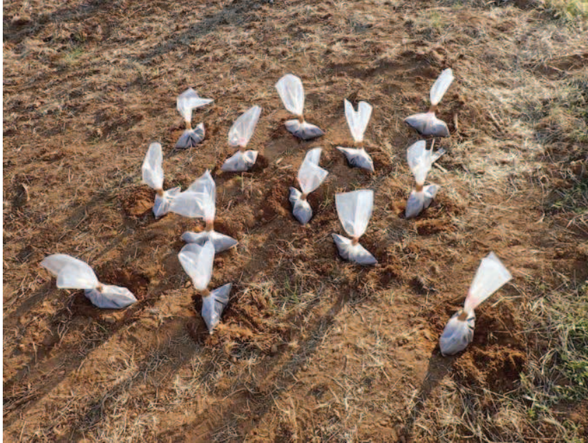
Figure 4.11: Soil samples collected at a natural calibration site to be characterized via laboratory gamma-ray spectroscopy measurements.
