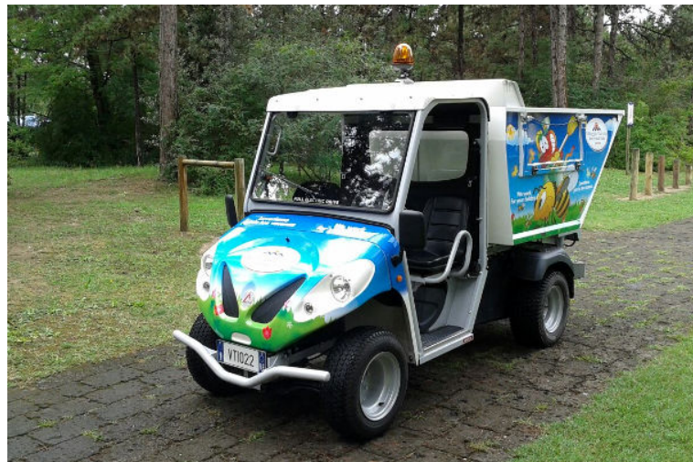
Figure 6-12: small electric vehicles (BWC WM 5.2) with a capacity of 655 kg (2.200 liter) has an autonomy of 70 km and a max speed of 35/44 km/h
