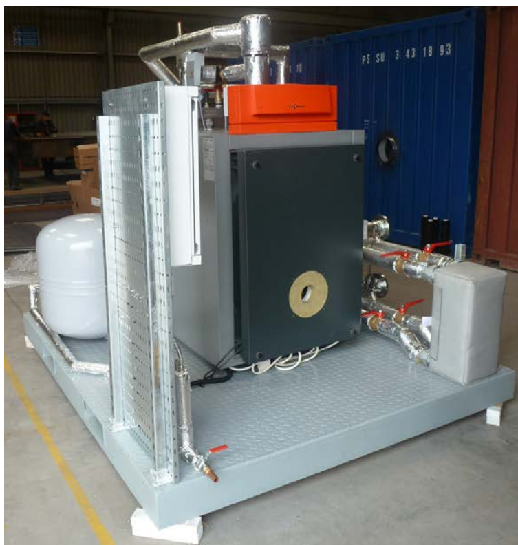
Figure 6-25: boilers (PU BU 1.1) produces hot water
