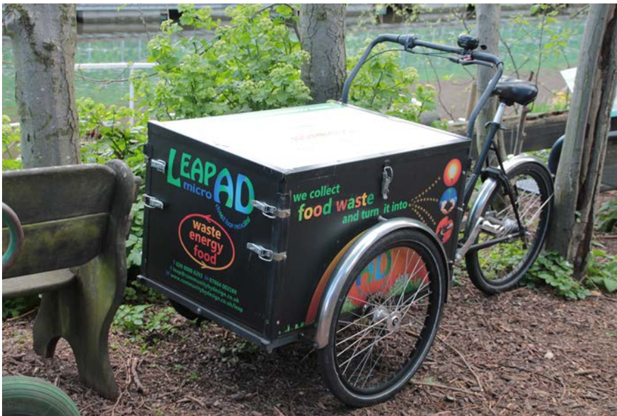
Figure 6-10: bike cargo (BWC WM 5.1) is a small cycling vehicle that collect up to 100 kg of food waste with an average speed of 15/20 km/h
