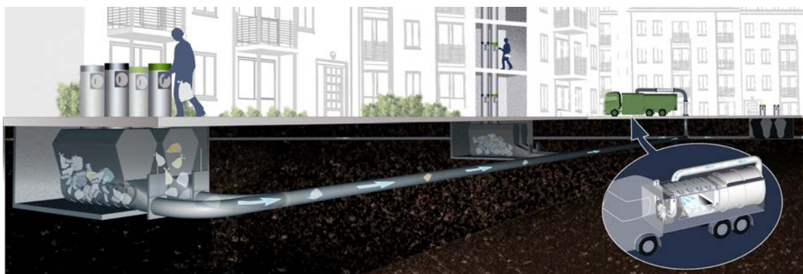
Figure 6-15: pneumatic collection mobile station (BWC FM 5.5.4)
