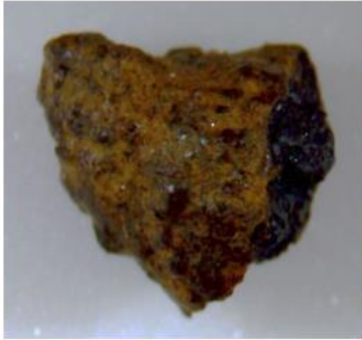
Figure 9.3: Sample DWKA/RCS1/18 (4000microns): Rock fragment composed of black mineral stained with iron oxide [Goethite + Hematite].
