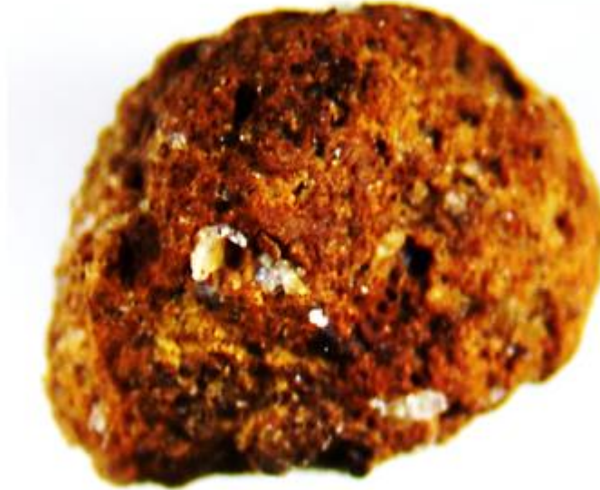
Figure 9.7: Sample ARRI PHI/RCS1/18 (+4000microns): Iron Oxide ball enclosing fine quartz grains
