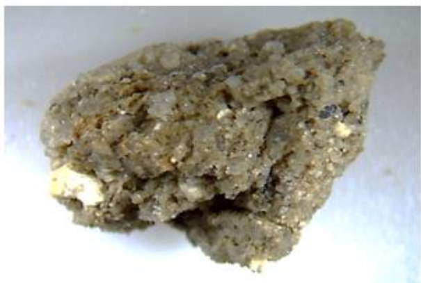
Figure 9.6: Sample DRDA/RCS1/18 (+4000microns): Multiple quartz grains cemented together to form a single grain.
