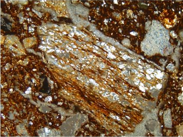
Figure 6.16 C: Sample no. 8, Grit tempers of rock fragments (Feldspars enclosing finer parallel oriented grains of feldspar with iron oxide strings).
