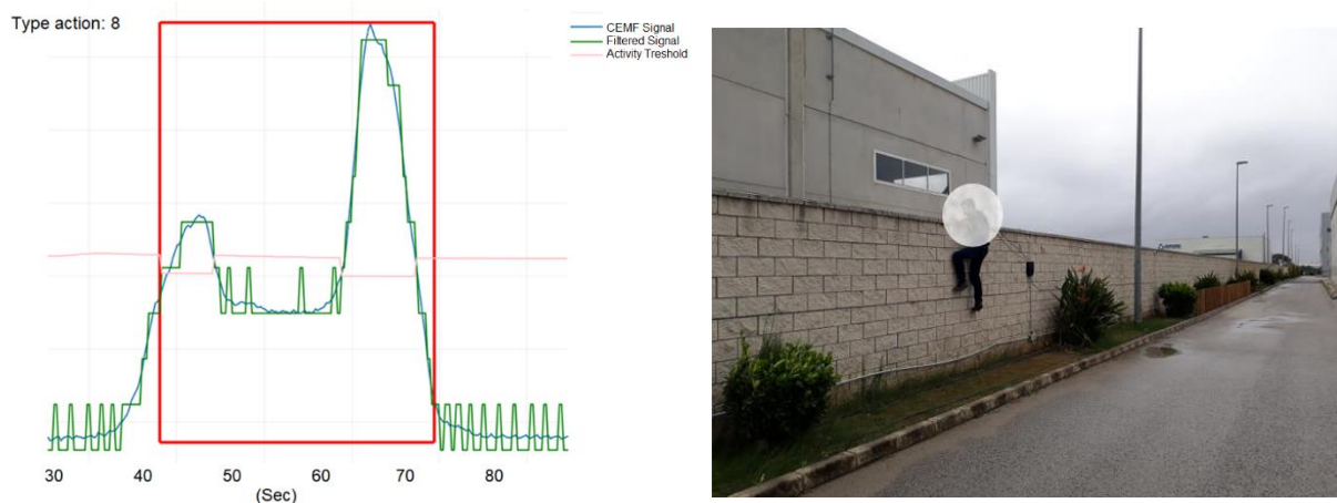
Figure 29. Image validating of a CEMF event in the field.
