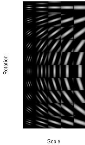
Figure 4. 2D Gabor wavelets for 5 different scales and 10 different rotations
